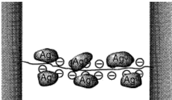
The scheme of assembling DNA-templated metallic nanowire with electrodes (10)**
