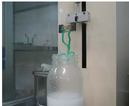
Deep coating procedure
