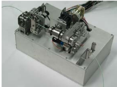
Linear Stepping Mechanism (LSM) for catheter control (2003)
