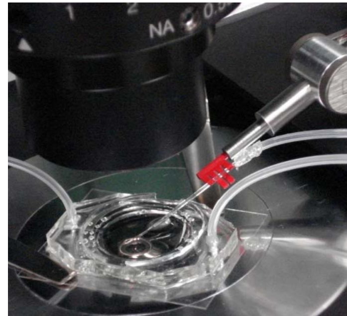
Insertion of the micropipette to the semi-closed microchip
